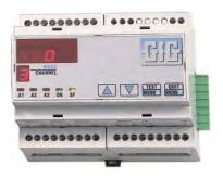
Each controller has four relays which can be switched normally open or closed. These relays can activate external alarm devices, or switch on ventilation, for example. Using an internal **plug connector** (bus system), a number of controllers can be combined as an option. A common power supply and transmission of multiple alarms can therefore be achieved without the need for additional wiring.
