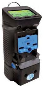
optional **Ex certified LED flashlight**, which is built into the battery pack. Either rechargeable NiMH battery packs or alkaline battery packs can be used. A **variety of chargers** are also available, so that charging over a range of voltages from 12/24Vdc, 115VAC to 230VAC is possible. The charger is also the platform for data transfer from the Microtector II to PC.
