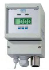
with integrated sounder and alarm LEDs. Configuration and calibration use simple menus accessed via the 3 keys on the front panel. Operation and maintenance are straightforward. The AutoCal program ensures an automatic calibration of the sensor to a known concentration of test gas. The GMA36 pro uses smart, plug and play electro-chemical sensors that can be easily exchanged.
